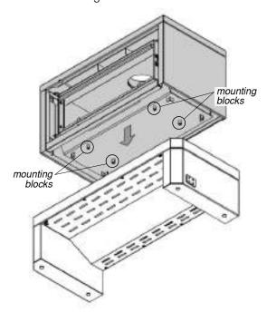
Align the mounting blocks with the holes in the top face of the bench. The holes to be used are outlined below.
