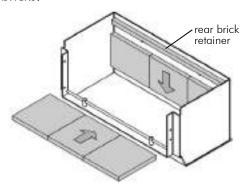
The side firebricks have an angled cut on the top edge. Place these firebricks into the firebox so that the shorter edge is at the rear of the firebox and the longer edge is at the front.
