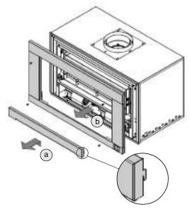
b. The fascia body is attached by 4 screws. Remove these screws and set them aside. Carefully slide the fascia forward to remove.
