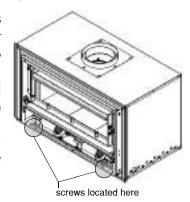
Slide the heater body forward to allow for the cladding to fit in between the zero clearance casing and the heater body.
