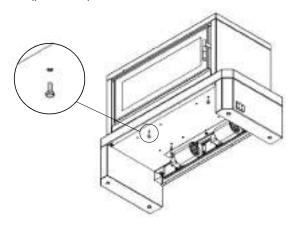
Replace the cover panel and fix into place with the 8 screws.
