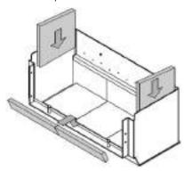
Next, place the rear baffle holder into the firebox. This sits on top of the side firebricks at the rear of the firebox. There are two locating holes in the holder that sit over pins in the rear of the firebox.
