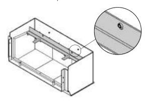
Place the front baffle holder into the firebox. This sits on top of the side firebricks towards the front of the firebox. There are two locating holes in the holder that sit over pins at the front of the firebox.
